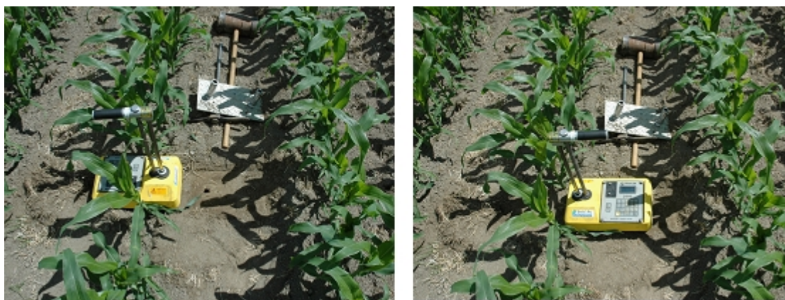
Fig. 4. Position of Gauge for in-row (left) and inter-row (right) Soil Density-Moisture measurements
