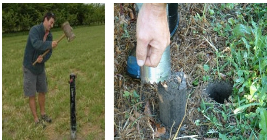
Fig. 5. Sampling using bulk density soil corer: Installation (left) and extracted core (right)
