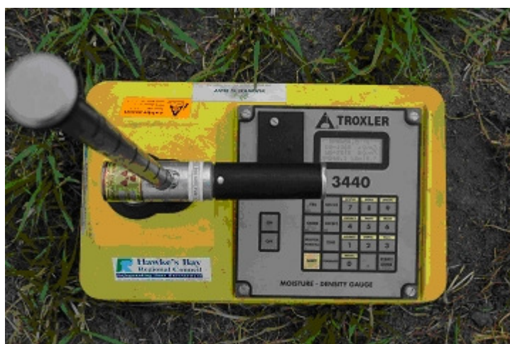
Fig.1 View of Troxler 3440 Neutron Densometer with source set at 300mm soil depth
