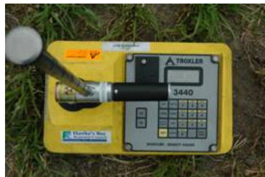
Fig.1 Top view of Troxler Moisture-Density Meter
