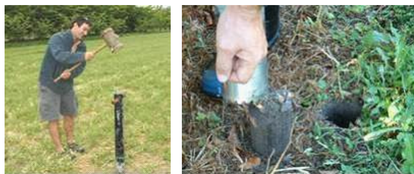
Fig. 5. Sampling using bulk density soil corer: Installation (left) and extracted core (right)
