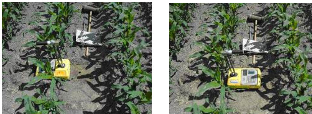
Fig. 4. Position of Gauge for in-row (left) and inter-row (right) Soil Density-Moisture measurements in a strip tillage versus full cultivation trial growing maize for silage.
