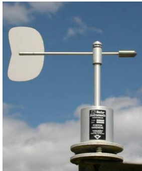
A windvane used for measuring wind direction
