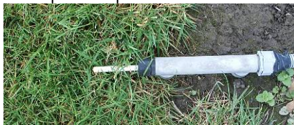
Screened and unshielded temperature sensors - grass minimum temperature probe shown below
