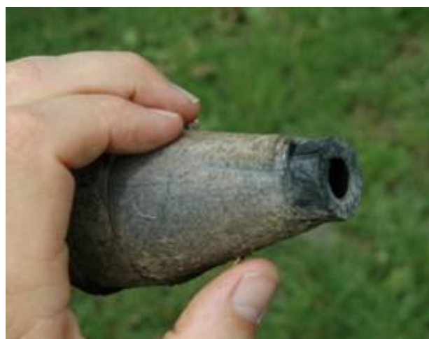
Figure 4. Splash plate fitted to end nozzle to widen spread Figure 5. Rubber nozzle crimped & cut to increase footprint
