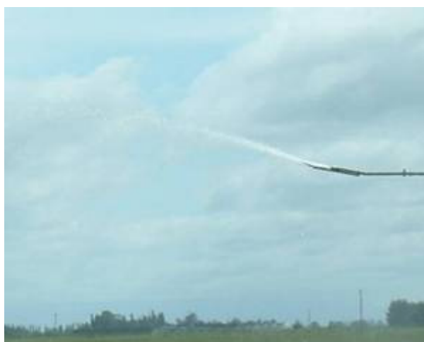
Figure 4. Splash plate fitted to end nozzle to widen spread Figure 5. Rubber nozzle crimped & cut to increase footprint
