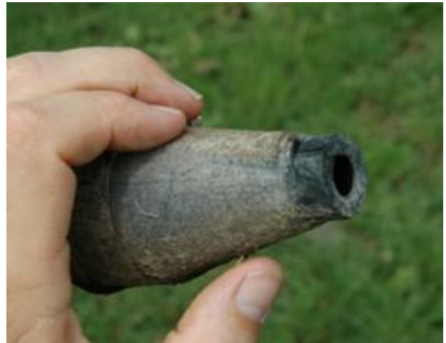
Figure 3. Splash plate fitted to end nozzle to widen spread Figure 4. Rubber nozzle crimped & cut to increase footprint
