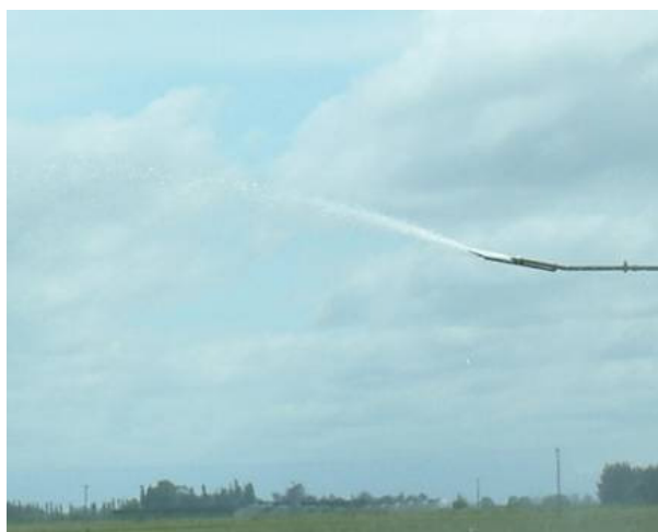
Figure 3. Splash plate fitted to end nozzle to widen spread Figure 4. Rubber nozzle crimped & cut to increase footprint
