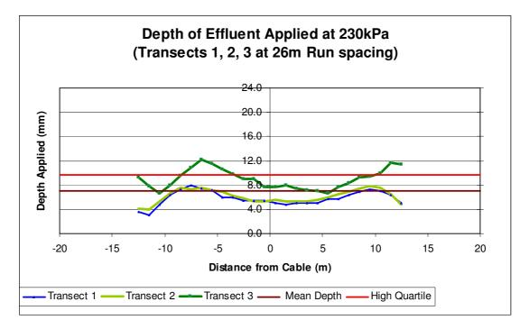
Figure 2. Effluent application pattern of three transect along a single run, measured at 230kPa pressure and full machine speed with calculated overlapped pattern based on 26m run spacing
