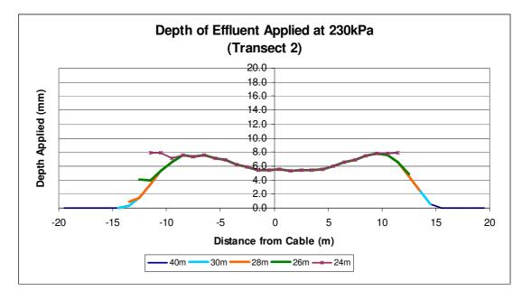
Figure 3. Effluent application pattern measured at 237kPa pressure with machine speed standardised: calculated overlapped pattern based on 40 (no overlap), 30, 28, 26 and 24m run spacings
