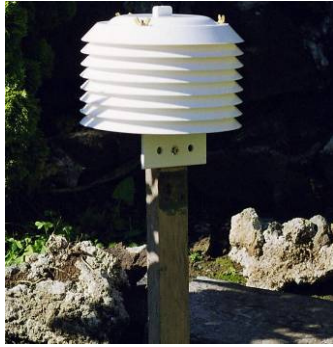
Plastic stacked plate sensor screen sold for use with Tiny Tag loggers.
