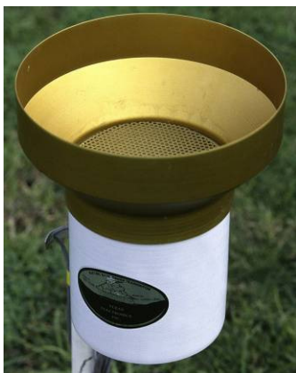
Tipping bucket rain gauge with wide collection funnel used for 0.1mm tipping increments. The tipping mechanism is shown below.
