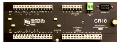
A multi channel programmable data logger (Campbells CR10).
