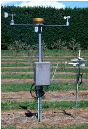
Two electronic weather stations, linked to telephone modems and fitted with a range of sensors.
