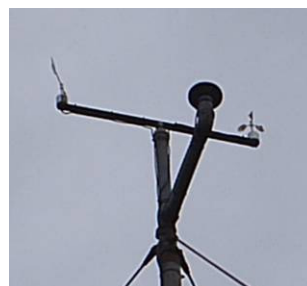
Cup anemometer used to measure wind run. Shown on a met mast below with wind direction and solar radiation sensors.
