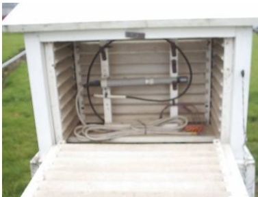
The wooden Stevensons screen (small version shown) is the world standard screen for meteorological observations
