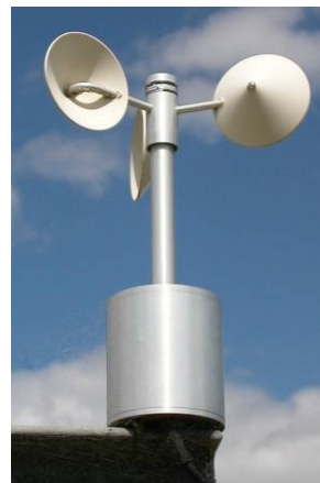
Cup anemometer used to measure wind run. Shown on a met mast below with wind direction and solar radiation sensors.
