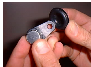
The low cost Ibutton Thermochron temperature logger
