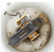
Tipping bucket rain gauge with wide collection funnel used for 0.1mm tipping increments. The tipping mechanism is shown below.
